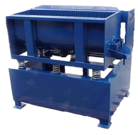
Designed to *reduce cycle times* and produce clean finished parts. The 120 volt, 1.5 horse power electric motor, energizes a sub-shaft that powers up the main eccentric weighted shaft producing the energy to move erratic shapes of media into the flowing motion which deburrs or polishes your parts *in house*.
