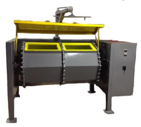
This heavy duty industrial machine has the capacity to ball burnish, polish or deburr very large parts or large volumes of medium sized product and is powered by a heavy duty motor and gearbox that directly drives the barrels with a variable speed drive unit which forces the media flow over your parts to create beautiful finishes.
