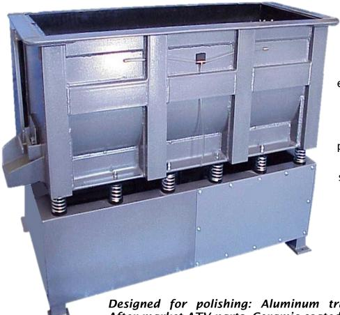
The 220 volt, 5 hp electric motor, energizes a sub-shaft that powers up the main eccentric weighted shaft producing the energy to move erratic shapes of media into the flowing motion uniformly deburring or polishing your parts.
