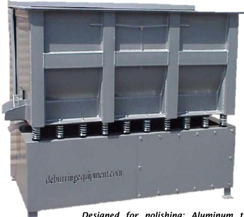
The 220 volt, 7.5 hp electric motor, energizes a sub-shaft that powers up the main eccentric weighted shaft producing the energy to move erratic shapes of media into the flowing motion uniformly deburring or polishing your parts.
