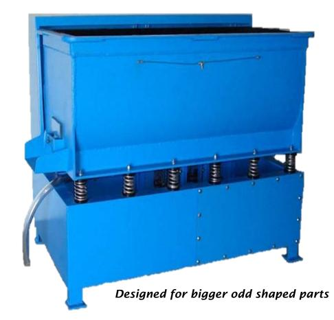
8 Cu. Ft. machine Tub: 56" x 18" x 18" Footprint: 65" x 35" x 42" 220 volt, 2 horse power, 3 phase motor\* Lining – hot poured urethane (industry standard) 5 gal. compound bucket, recirculation pump & pump hanger Holds 350 lbs. ceramic media or 200 lbs. plastic media (plus parts) \*magnetic starter not included
