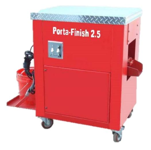
Portable on 4 urethane casters. Stainless Steel Sound Cover 5" Media Discharge door 120 volt, 1 horse power motor Lining – hot poured urethane (industry standard) Easy access exterior 5 gal. compound bucket & recirculation pump
