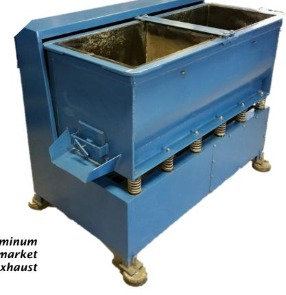
Designed for polishing: Aluminum transmission cases, After market ATV parts, Ceramic coated exhaust systems
